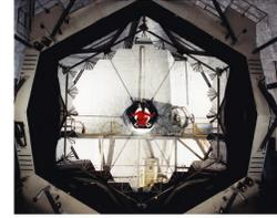
Segmented 10-meter mirror of a Keck telescope
