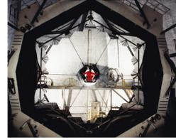
Segmented 10-meter mirror of a Keck telescope
