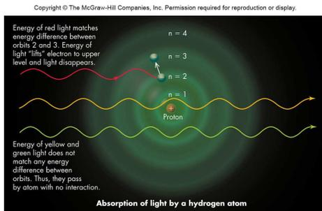
Absorption of light by a hydrogen atom
